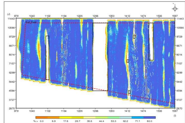
Figure 1: Limited offset coverage plot, with application of hole detection, output from the Integrated Navigation System onboard the vessel
