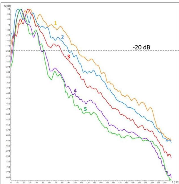
Figure 3: Amplitude spectra measured in the target windows shown in Figure two, demonstrating the effect of the earth's attenuation on the frequency content of seismic targets with depth.
