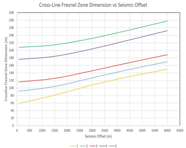
Figure 4: Cross-line Fresnel Zone dimensions plotted as a function of seismic offset and used to define illumination requirements for each target.
