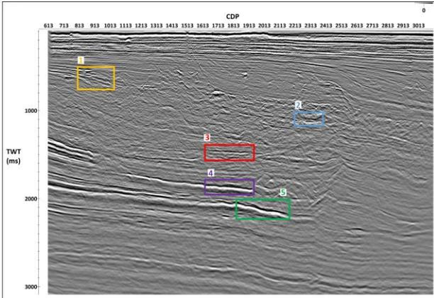
Figure 2: Example seismic section, with application of demultiple, deghosting (broadband), and prestack migration, demonstrating selection of target windows for measurement of frequency spectra.
